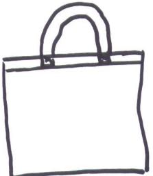
Step 5. Attach your straps! With your bag inside out, each strap will lay over the top edge 1". Stitch around the edge of the strap over the bag in one continuous square stitch. For added durability you can also stitch an X across the square from corner to corner. Repeat for each end of each strap.
